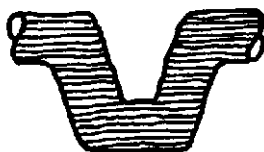
Bar Stock Grain flow broken by machining
