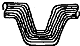
Forging True grain flow
